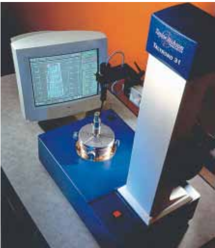
圆度仪(英国) Roundness measurement instrument (UK)
